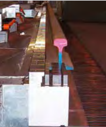
A ) Milling of the switch and stock rails to length 2 x 24 m
