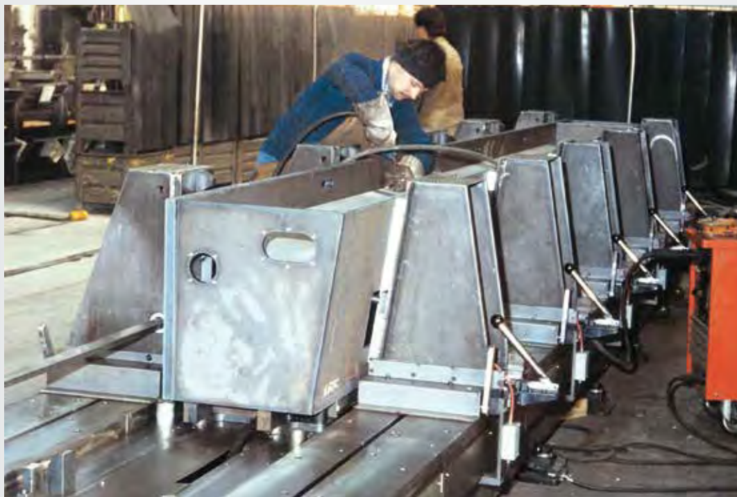
Magnetic welding fixture in a special execution. For details, see below.
